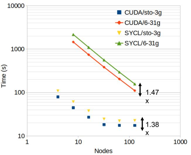
Strong scaling – Contribution of timings in seconds for (T) kernel on ALCF Polaris, each node with 4 Nvidia A100 40 GB. Nodes: 4, 8, 16, 32, 64, 128
